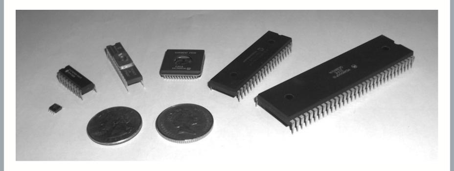
From left to right: PIC 12F508, PIC 16F84A, PIC 16C72, Motorola 68HC05B16, PIC 16F877, Motorola 68000
